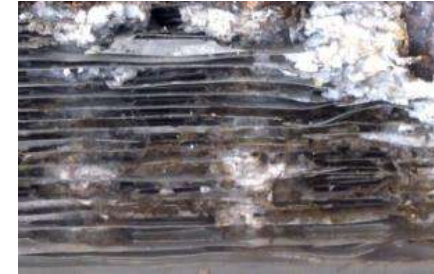
Unprotected coil after 4000 hours salt spray test
