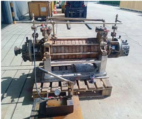
Hydro- Test Repaired Pump
