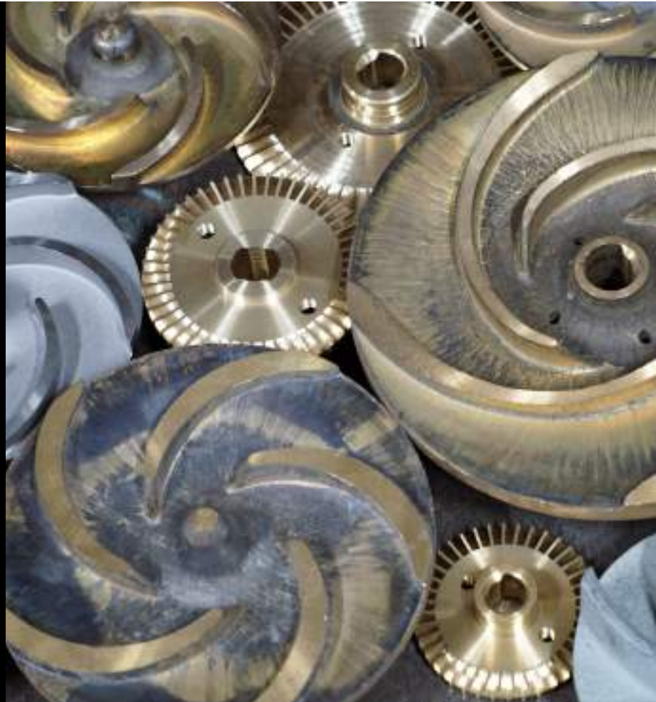
NON-KBL MAKE R55 MOC PUMP MODEL – 125-80- 250 SCANNED WITH 3D PRINTER WORN OUT R55 IMPELLER
