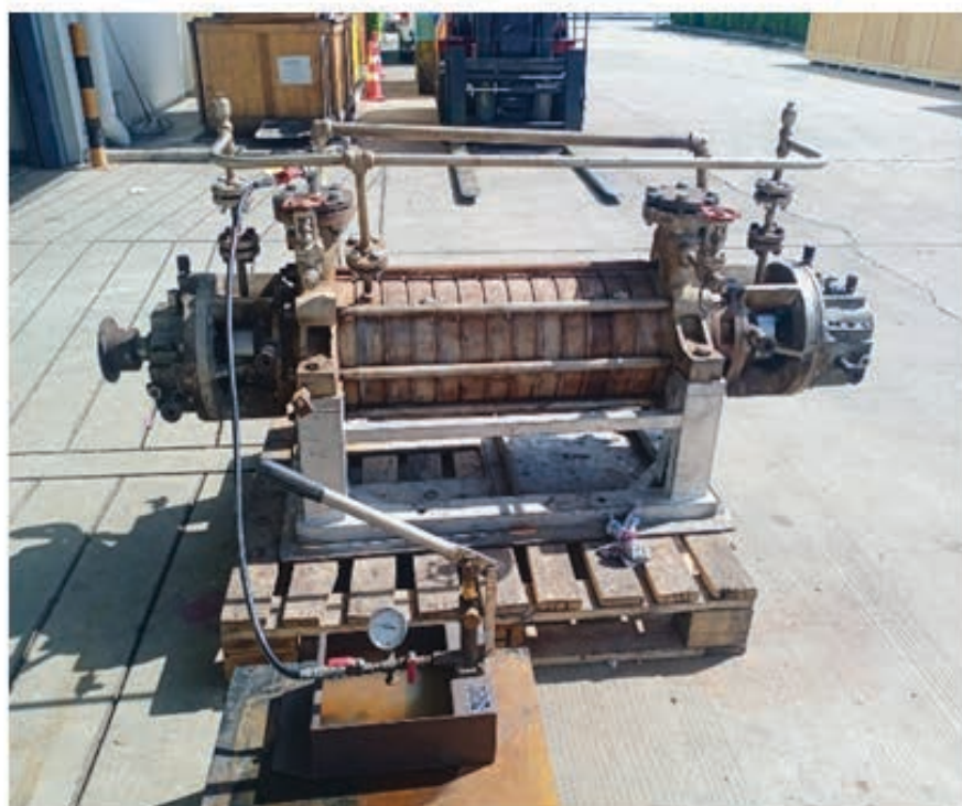
Hydro- Test Repaired Pump
